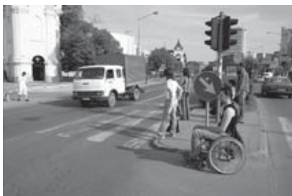
Islands are not cut for wheelchair users
